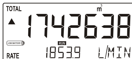
Fig. 4: Example of low-battery alarm.
