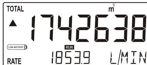
Fig. 4: Example of low-battery alarm.
