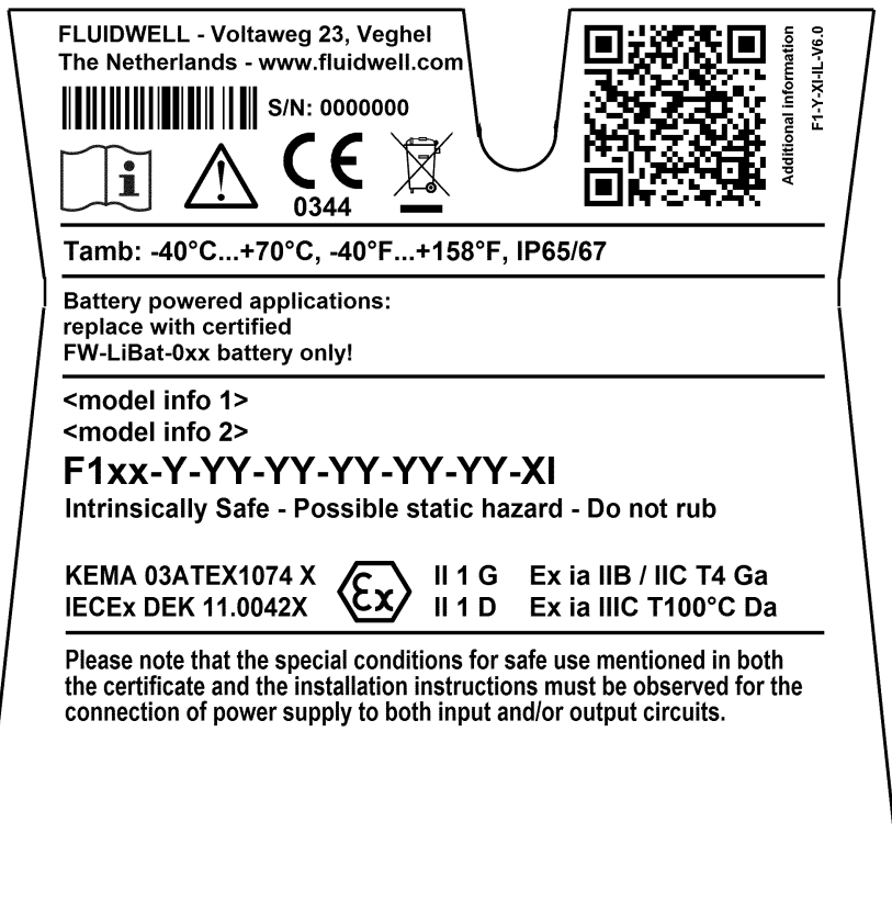
Fig. 24: Label information - Intrinsically safe application (typical)
