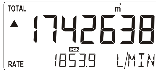
Fig. 3: Process information (typical)
