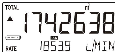
Fig. 4: Example of low-battery alarm.
