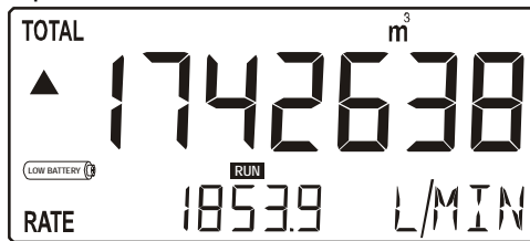
Fig. 4: Example of low-battery alarm.
