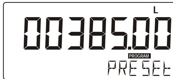
Fig. 3: Example displayed information during programming preset value.
