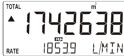
Fig. 3: Process information (typical)
