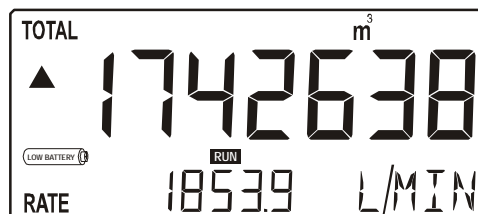
Fig. 4: Example of low-battery alarm.
