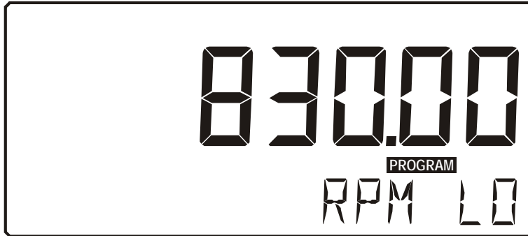
Fig. 4: Example of display information during programming minimum engine speed.
