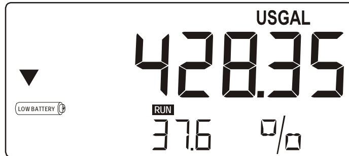
Fig. 5: Example of low-battery alarm.
