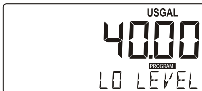
Fig. 4: Example of display information during programming minimum level.
