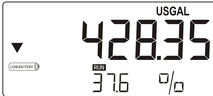
Fig. 5: Example of low-battery alarm.
