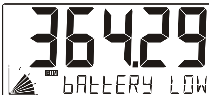
Fig. 4: Example of low-battery alarm.
