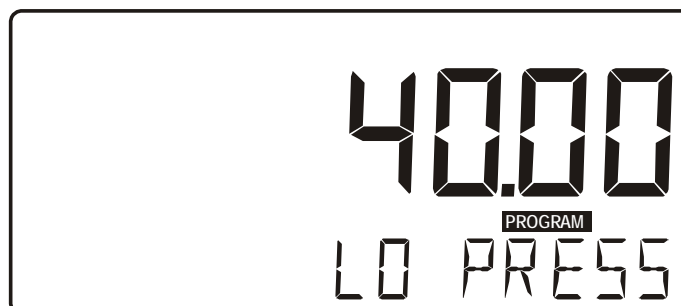
Fig. 4: Example of display information during programming minimum pressure.
