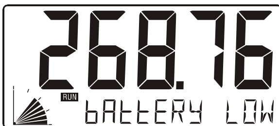
Fig. 4: Example of low-battery alarm.
