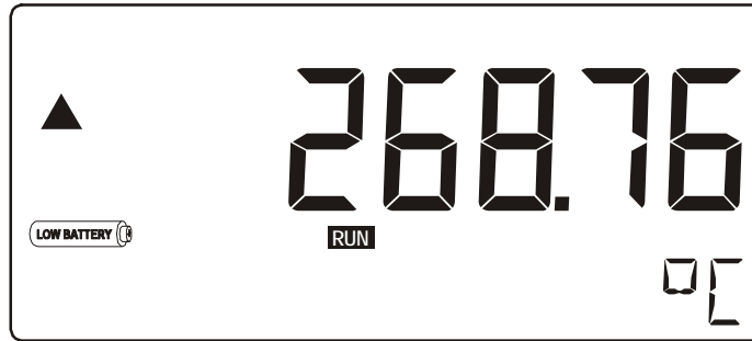
Fig. 5: Example of low-battery alarm.
