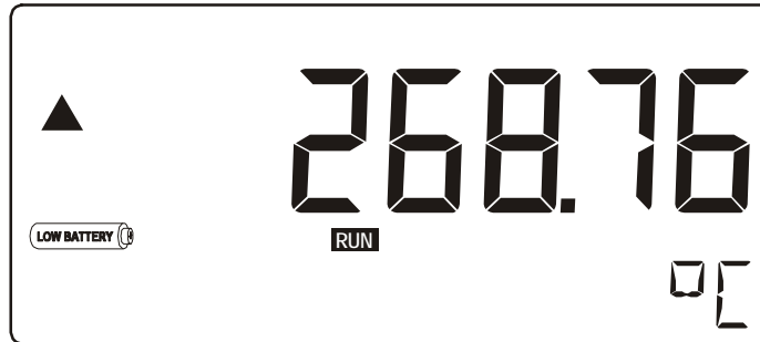
Fig. 5: Example of low-battery alarm.
