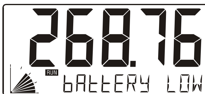
Fig. 4: Example of low-battery alarm.
