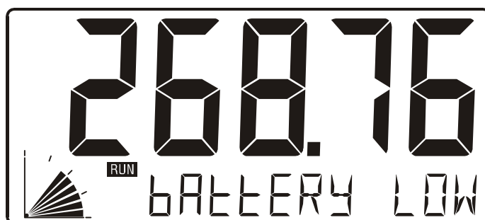
Fig. 4: Example of low-battery alarm.
