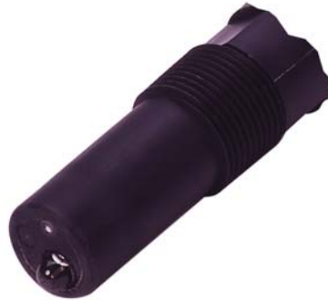
Figure 13. PH10-2 Electrode, Domed Bulb without Protective Guard
