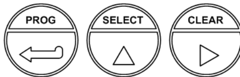
Fig. 2: Control panel, optical keys.
